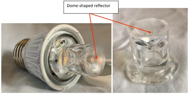
(photographs of TCP A19 Omni Directional Lamp with outer glass bulb removed, showing dome-shaped reflector above LEDs, and of dome-shaped reflector itself).
