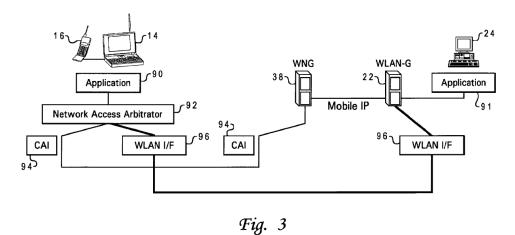
Fig. 3 is a schematic diagram of a wireless data communication system for seamless roaming between wireless networks.
