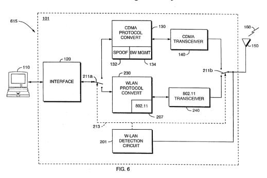
Figure 6 is a block diagram illustrating the subscriber unit.
