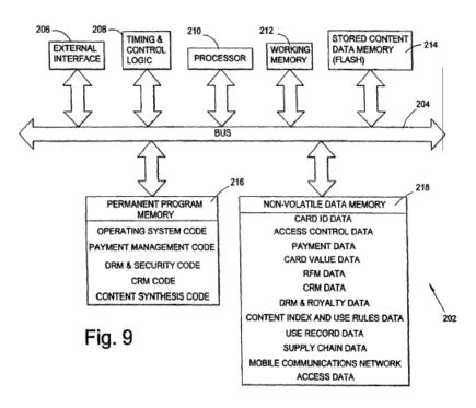
Figure 9 is a schematic diagram of the components of portable data carrier 202. Portable data carrier 202 is shown as a "smart Flash card." *Id.* at 17:6–8.
