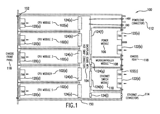
As shown above in Figure 1, computer network appliance 100 includes CPU modules 102(a)–(e), power module 106, microcontroller module 108, and Ethernet switch module 110 connected to the backplane 104 via hot swap connectors. *Id.* at 3:18–23, 32–37. A chassis 150 encloses backplane 104
