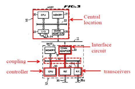
As shown in annotated Figure 3 of Tymes above, host processor 10 (central location) is connected to base station 13 (a device for communication information) via link 11. Base station 13 includes CPU 30 (controller), which is coupled to *RF transceiver* 34, communication adapter 33 (interface circuit), and memory 31, via local bus 32. *Id.* at 6:63–7:35. RF transceiver 34 in base station 13 is connected to antenna 35 for receiving and transmitting data to and from remote units 15. *Id.*
