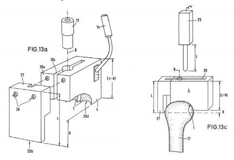
Figures 13a and 13c schematically show an individual template 4 for the preparation of the seat for a knee-joint head prosthesis. *Id.* at 30.
