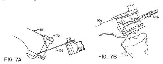
Figures 7A and 7B present a lateral view and a perspective view of a cutting guide for making final femoral cuts. *Id.* at 3:39–40.
