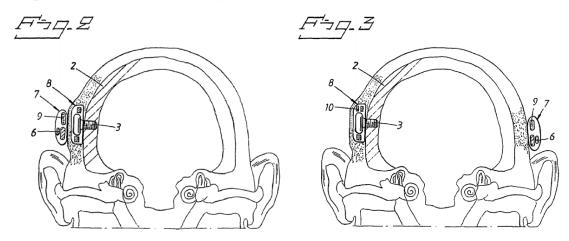
Figures 2 and 3 depict schematic views of a skull in which a hearing aid is partially implanted. *Id.* at 2:34–39, 3:9–11. As shown in Figure 2, implantable part 8 includes a vibrator, while external part 7 includes microphone 6 and battery 9. *Id.* at 3:9–12. "[P]ower is transmitted to the implanted part 8 of the hearing aid by means of induction." *Id.* at 3:12–14.
