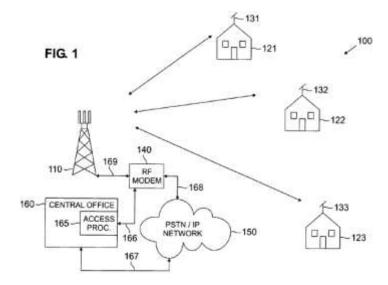
Figure 1 illustrates fixed wireless access network 100, which comprises transceiver base station 110 that transmits forward channel broadband signals to subscriber premises 121, 122, 123, and antennas 131, 132, and 133. *Id.* at 11:57–12:6. Transceiver base station 110 is coupled to RF modem shelf 140, which converts baseband data traffic received from external network 150 to RF signals transmitted in the forward channel to subscriber premises 121, 122, and 123. *Id.* at 12:15–22.
