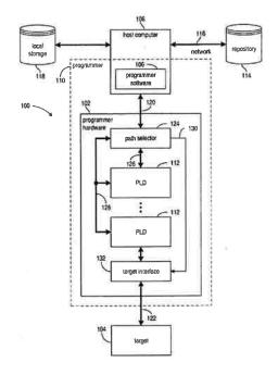
Figure 1 illustrates the programmer hardware implemented with one or more PLDs 112. Ex. 1007, 3:44–46. The programmer hardware receives configuration data on lines 120. *Id.* at 3:35–37.
