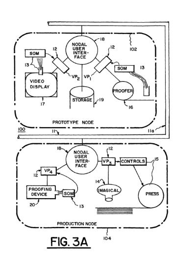
Figure 3A depicts prototype node 102 connected to production node 104 via network 11. *Id.* at 11:54–12:6. Prototype node 102 allows a user to interface with a node to perform pre-publishing functions and to input digital color image data. *Id.* at 12:6–43. Using prototype node 102, a user may design a page layout and define color preferences for rendering of color image data. *Id.* Production nodes 104 control production of a rendering
