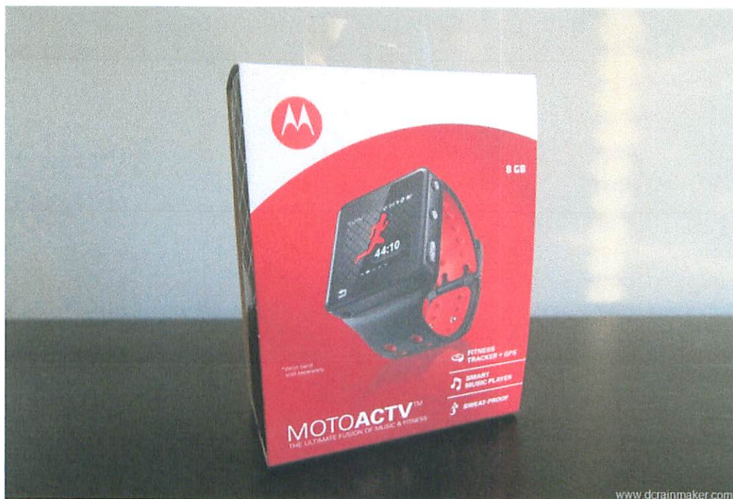
FIG. 1: The MOTOROLA MOTOACTV™ device includes an internal accelerometer to track steps taken by its wearer. The Kit includes a CLIP that may be attached to a person's belt, shirt, shoe, etc. to accurately record activity metrics in accordance with steps taken, etc.
