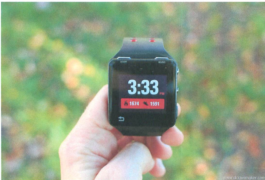
FIG. 2: A MOTOROLA MOTOACTV™ activity tracker displays steps taken based on operation of its internal accelerometer. As show, the person has taken 1591 Steps by determining foot action including when a person's foot is off the ground in the air during a step, a jump, etc.
