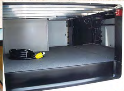
Huge pass-through basement with fold-down bulkhead wall to separate and organize cargo.
