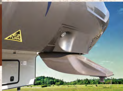
Unique XLT Extended Hitch Pin for maximum turning clearance on short bed trucks; optional ABS Hitch Cover.
