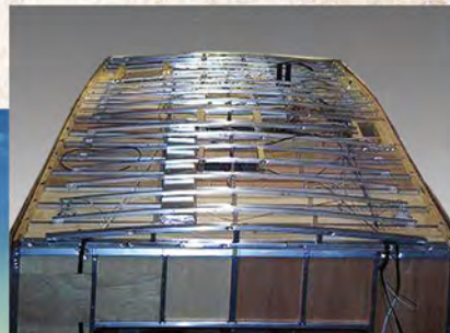
Welded square-tube aluminum frame is strong, lightweight and durable.
