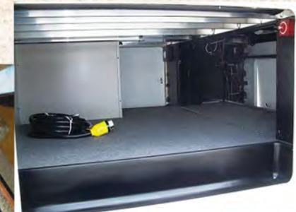
Huge pass-through basement with fold-down bulkhead wall to separate and organize cargo.
