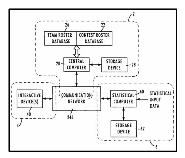
'862 patent, Fig. 1B (showing the implementation of the '862 patent system arose from receiving user data over a communications network, such as the internet, including through a website).
