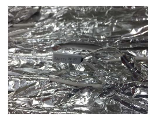
Element f: an electrical cord covered by a metal spring that is electrically coupled to the low wattage heating wire.
