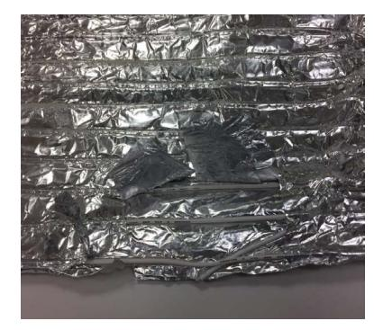
Element c: a foam layer adjacent to one side of the foil packet wherein the foil packet is electrically grounded and the foam layer is fire retardant and is glued to one side of the foil packet;
