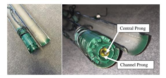
43. Claim element 1(d) of the '416 Patent recites "a second power distribution subsystem disposed within an inner void of a second trunk section of the plurality of tree trunk sections, the second power distribution subsystem comprising a female end, the female end having a central void and a channel void."
