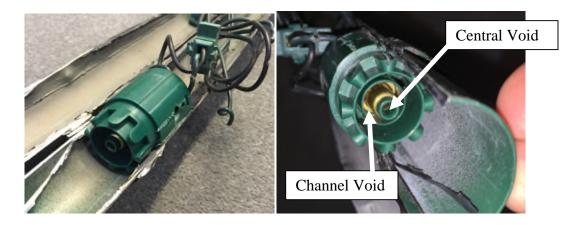
95. Claim element 1(e) of the '495 Patent recites "the central void having a central contact device disposed at least partially therein, and the channel void having a channel contact device disposed at least partially therein, the channel contact device disposed around the central void, and the central contact device and the channel contact device configured to conduct electricity."
