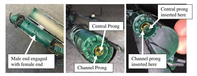
49. Claim element 1(g) of the '416 Patent recites "wherein, when the central prong engages the central void, the central prong pushes a spring activated contact section of the one or more spring activated contact sections causing the spring activated contact section to press against the central prong to maintain electrical contact between the central prong and the contact device."
