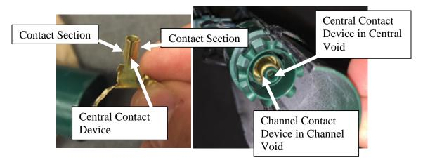
72. Claim element 1(f) of the '810 Patent recites "wherein the central prong of the male end is configured to engage the central contact device of the female end and the channel prong of the male end is configured to engage the channel contact device of the female end to conduct electricity between the male end of the first trunk section and the female end of the second trunk section."
