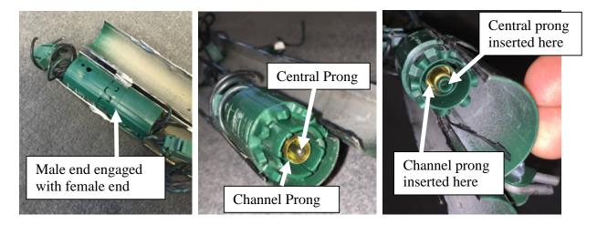
74. Claim element 1(g) of the '810 Patent recites "wherein, when the central prong engages the central contact device, the central prong pushes a spring activated contact section of the one or more spring activated contact sections causing the spring activated contact section to press against the central prong to maintain electrical contact between the central prong and the central contact device."
