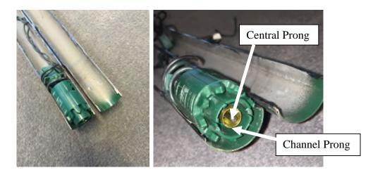
68. Claim element 1(d) of the '810 Patent recites "a female end of a second trunk section of the plurality of tree trunk sections, the female end having a central void and a channel void."
