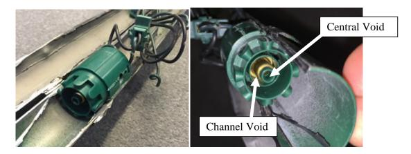
45. Claim element 1(e) of the '416 Patent recites "the central void having a contact device disposed at least partially therein, the contact device comprising one or more spring activated contact sections."
