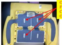
ONE OR MORE OPENINGS IN FORWARD LAYER IN FLUID COMMUNICATION WITH OPEN SPACE
