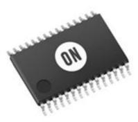
8. In general, integrated circuits, like those manufactured by ON Semiconductor, contain a single "chip" or "die" which is connected by wires to a number of "pins." The chip and pin-connections are encapsulated in a plastic case to form the packaged integrated circuit shown above. The pins allow the extremely small "chip" or "die" to be easily connected into a larger electronic system. An exploded view of an exemplary integrated circuit showing the "chip"/"die" and connected pins is shown below:
