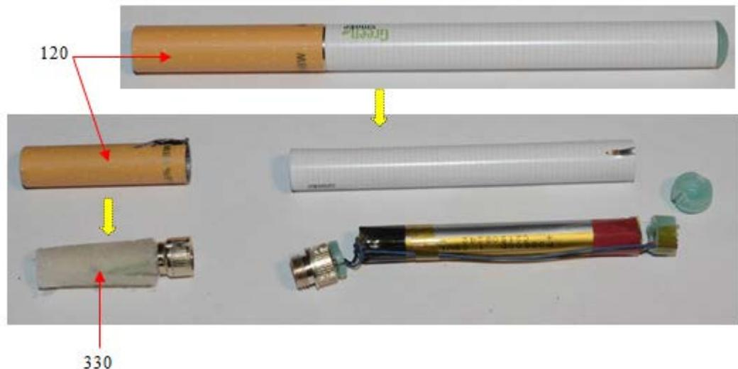
1           262. The GreenSmoke includes “the atomizer assembly [300] including a
