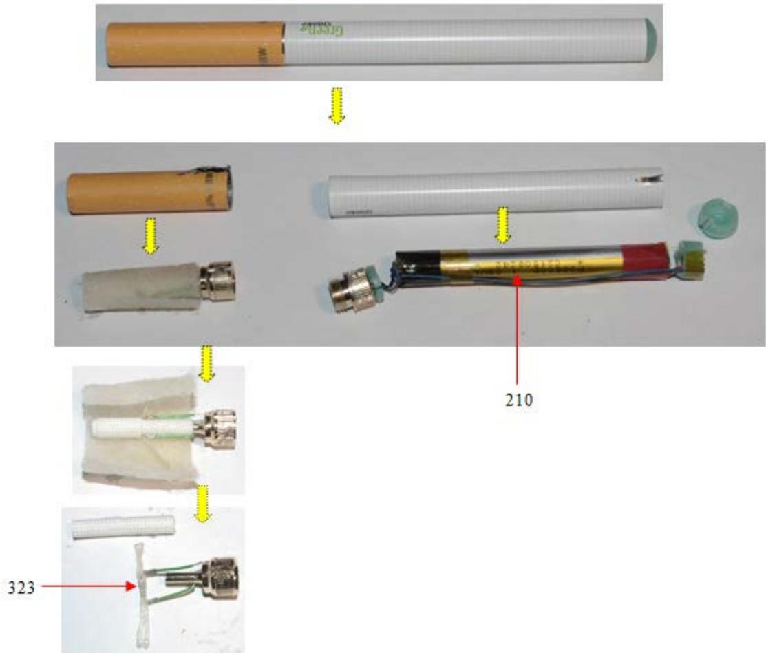
1           264. The GreenSmoke includes “an air flow path in the atomizer assembly
