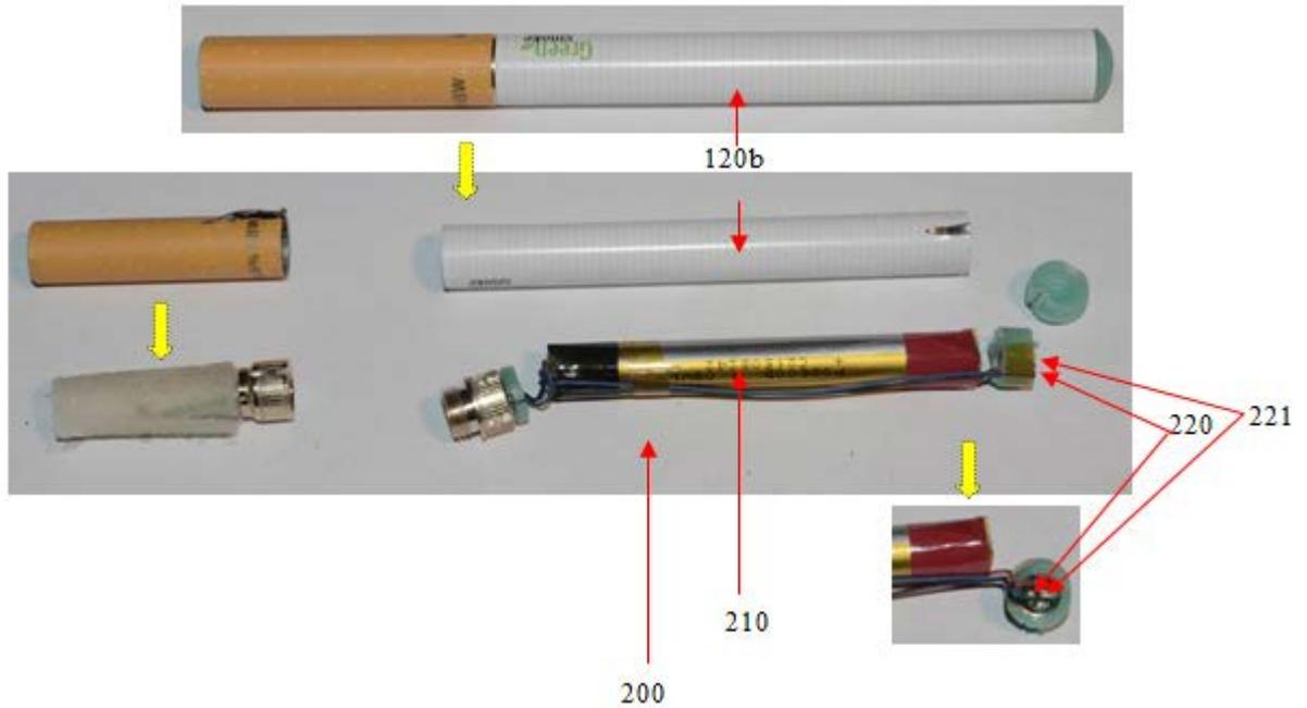
1           599. The GreenSmoke includes “a first screw thread electrode [160b] on the
