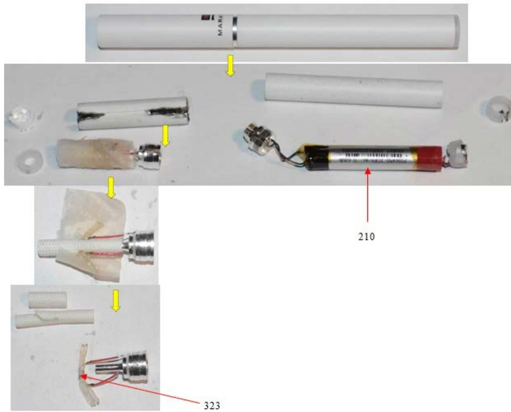
1           216. The MarkTenXL includes “an air flow path in the atomizer assembly
