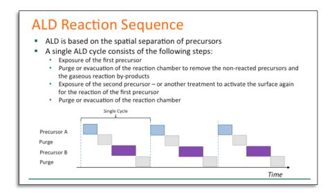
This is further illustrated by the process schematic, below, which shows a basic gas-flow
