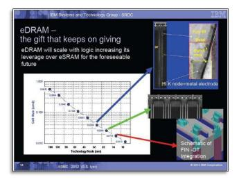
These trenches are further illustrated in the image below, which shows a scanning electron microscope image of a cross-section of eDRAM trench capacitors on the left and plan-view and
