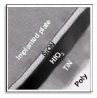
70. Further, Power8 server processors, such as those found in the Tyan Server, BSP010G70V8HR-2, include a hafnium silicate dielectric layer.<sup>56</sup> The image below is a transmission electron microscopy lattice image of a Power8 processor trench capacitor sidewall.
