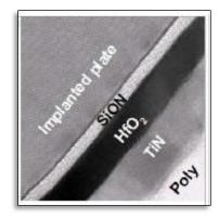
76. Further, Power8 server processors, such as those found in the Tyan Server, BSP010G70V8HR-2, include a hafnium silicate dielectric layer.<sup>65</sup> The image below is a transmission electron microscopy lattice image of a Power8 processor trench capacitor sidewall.
