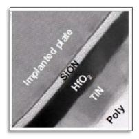
b. exposing a heated surface alternately to the vapor of one or more metal amides having an amido group selected from the group consisting of dialkylamido, disilylamido and (alkyl)(sily) amido moieties, and then to the vapors of water or an alcohol.
