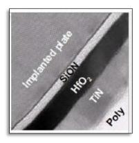
74. Further, Power8 server processors, such as those found in the Tyan Server, BSP010G70V8HR-2, include a hafnium silicate dielectric layer.<sup>61</sup> The image below is a transmission electron microscopy lattice image of a Power8 processor trench capacitor sidewall.
