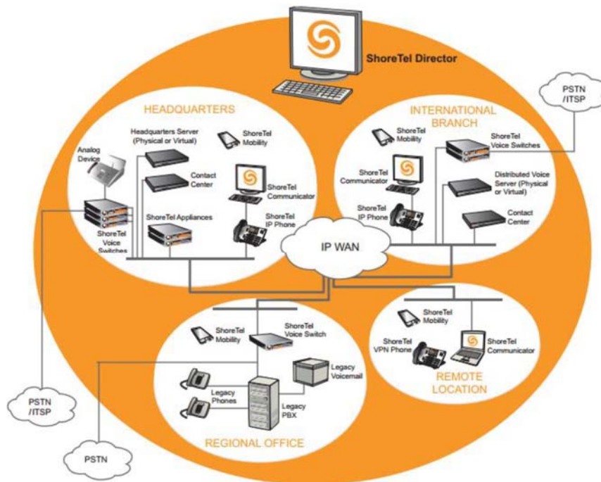
Figure 1: ShoreTel System with Single-Image Management
