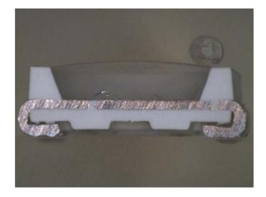
49. The cross-sectional x-ray image below illustrates that each of the leads can be considered as a top portion and a bottom portion having different planar shapes. The cross-sectional x-ray image also shows that the lead frame on the right as a fixing element with a space below the fixing element.
