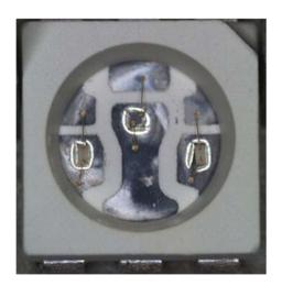
61. Reproduced below is an enlarged image of the portion of the printed circuit board from above after removal of the package. As shown by the green areas in the image below, the 3 LEDs are connected in series.
