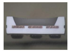
56. As can be seen in the below x-ray of the package, at least two terminals having different widths are shown in the group of terminals on the left and at least two terminals having different widths are shown in the group of terminals on the right.
