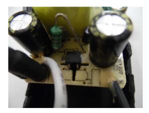
65. Returning to the first printed circuit board, a portion of which is depicted in the image below, a resistor labeled R8 is connected in parallel with the 3 LEDs provided in the package depicted above.
