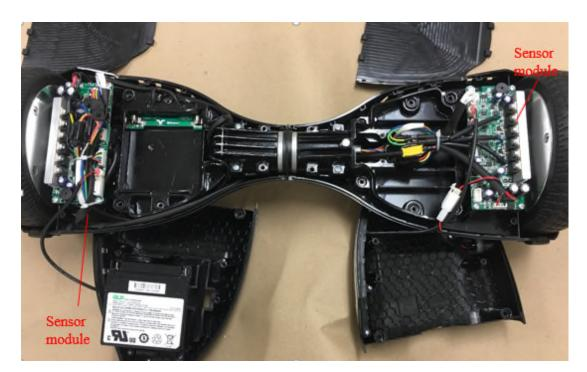
25. The Infringing Hoverboards contain a power supply fixed between the first bottom cover and the first inner cover. *See* Hovertrax 2.0 Owner's Manual, pg. 12 (part no. 13). The following image of the Razor 2.0 product depicts the battery, acting as the claimed power supply. The other Infringing Hoverboards also feature a substantially similar battery positioned similarly.
