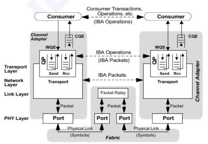
Figure 13 IBA Communication Stack
