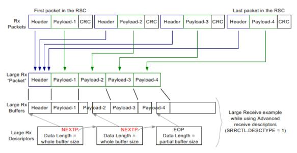
Figure 7-41 RSC Functionality (No Header Split)
