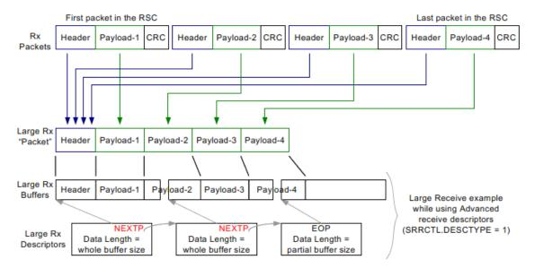
Figure 7-41 RSC Functionality (No Header Split)
