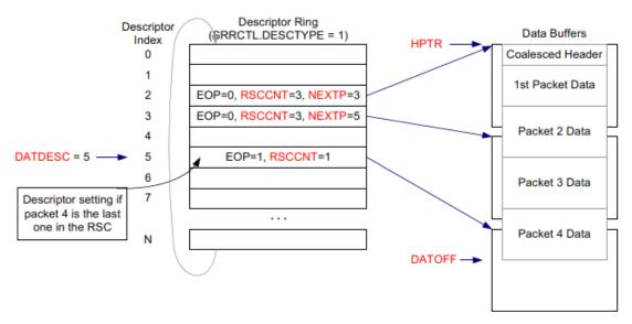
Figure 7-42 RSC Functionality (No Header Split)
