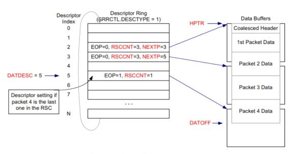
Figure 7-42 RSC Functionality (No Header Split)
