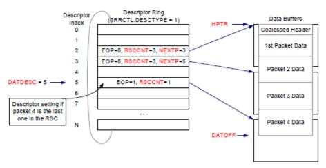
Figure 7-42 RSC Functionality (No Header Split)
