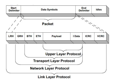
Figure 27 IBA Data Packet Format
