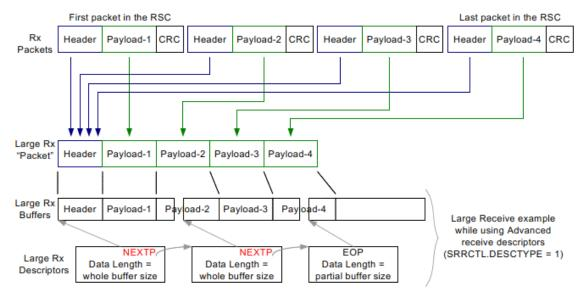
Figure 7-41 RSC Functionality (No Header Split)
