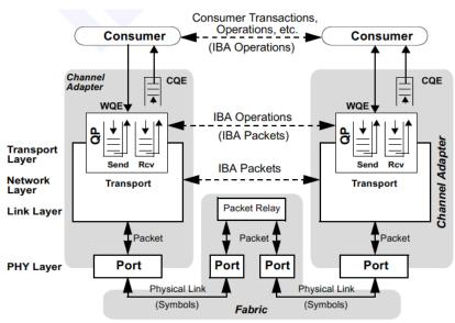
Figure 13 IBA Communication Stack
