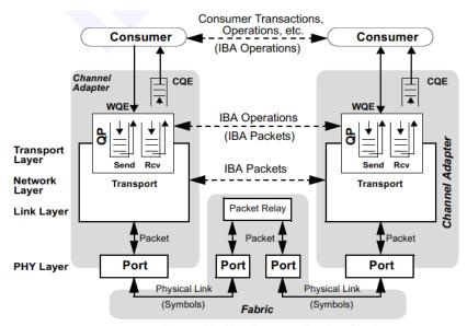
Figure 13 IBA Communication Stack
