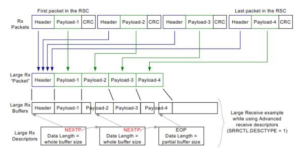
Figure 7-41 RSC Functionality (No Header Split)
