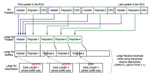
Figure 7-41 RSC Functionality (No Header Split)
