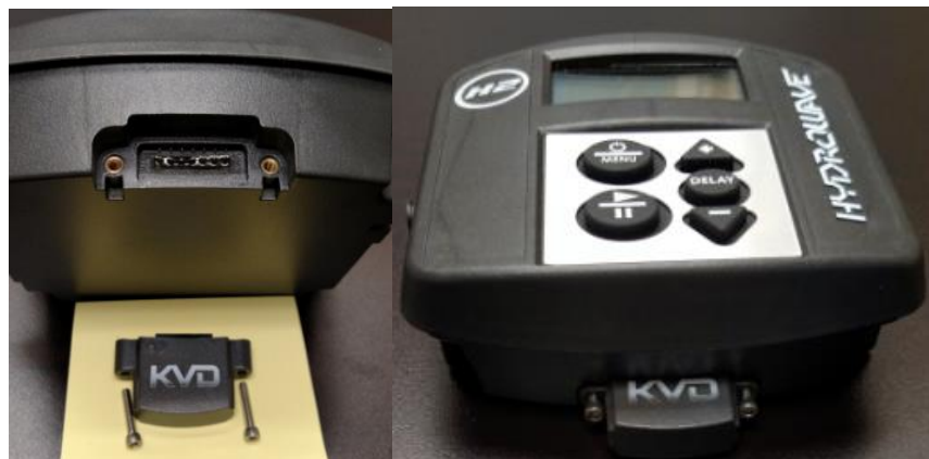
Hydrowave Expansion Module Installed in H2 System Expansion Port
