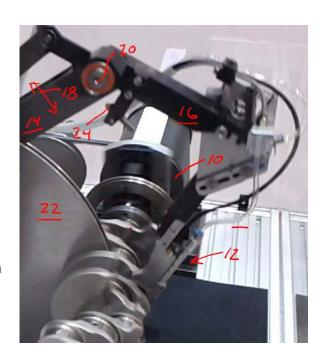
shown in the graphic above and to the right, the reference device 50 (see graphic below from a Jenoptik marketing document, with explanatory numerals added) is in contact with the cylindrical part. The DF500 device has a measuring device 12 movable with the reference
