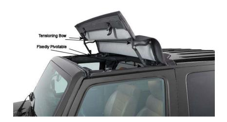
30. BesTop's Sunrider For Hardtop mechanism is displaceable between a closed position for covering the roof opening and an uncovering position as set forth in claim 6.
