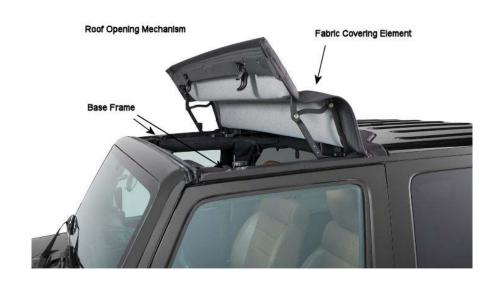
29. BesTop's Sunrider For Hardtop mechanism includes a tensioning bow fixedly pivotable with respect to the base frame as set forth in claim 6.
