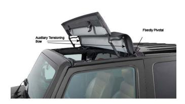
32. BesTop's Sunrider For Hardtop mechanism is configured such that the tensioning bow, in relation to a vertical longitudinal center plane of the roof, is on each of its two sides connected to the auxiliary tensioning bow via a coupling rod as set forth in claim 6.
