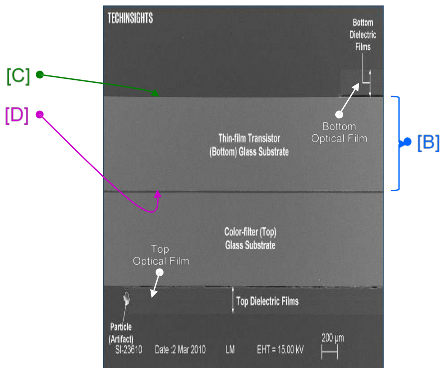
Cross Sectional View (a-a') of the LCD panel in Samsung LCD module, LTM 220M1-L01
