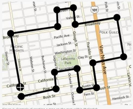
Figure 1: Example of creating a zone on the map within MyGeotab
