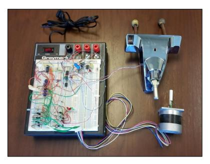
The experimental prototype (above) included a breadboard, bathroom sink faucet, and stepper motor.
