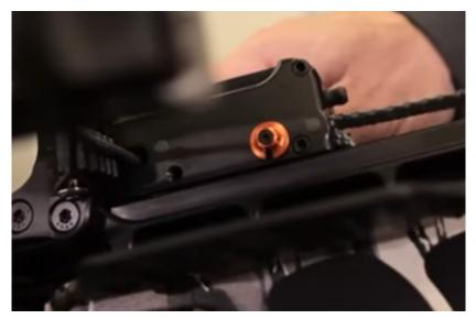
62. Within the image inserted near the top of the next page, captured from Defendant Ravin's instructional video named "Cocking Your Crossbow", Doug Guthrie of Defendant Ravin is seen operating a cocking crank to pull the cocking strap onto a winding spool until the movable bowstring release assembly is retracted and fully-cocked proximate to the trigger components:
