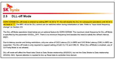
*SK Hynix DDR4 SDRAM Device Operation Manual*, SK HYNIX TECHNICAL DOCUMENTATION (June 2013), at 30 (highlighting added).
