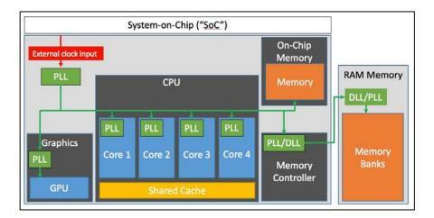
41. Modern SoC processors often also use additional system memory, which is provided as an external memory chip or module and interfaces with the processor through the processor's on-chip memory controller. The stylized figure above also shows an exemplary external memory module. Although there are many kinds of external memory that may be used, depending on the particular application, synchronous dynamic random access memory (or "SDRAM") is perhaps the most prevalent type.
