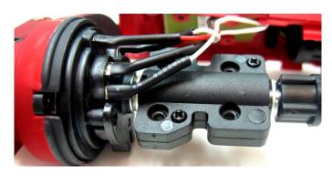
30. The following image of a dismantled Accused Product shows that the rotatable rod extends through the centers of both terminal discs and the contacts of both terminal discs circumscribe the rotatable rod:
