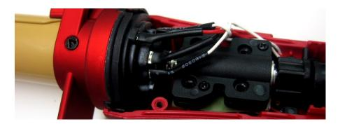
28. The following image of a dismantled Accused Product shows that the contacts on one of the terminal discs are bent upwardly and contacts on the other terminal disc are flat annular rings:
