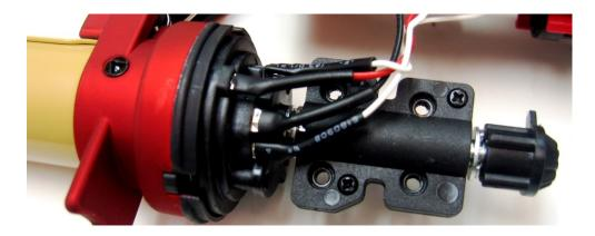
26. The following images of a dismantled Accused Product show that it has a first terminal disc fixed to the cylinder and includes concentric annular electrical contacts. The images also show the rod that is affixed to and rotates with the cylinder as described in ¶24:
