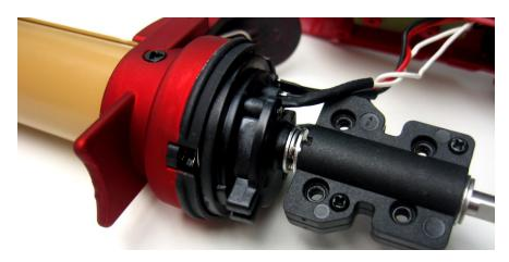
33. The following image of a dismantled Accused Product shows a thrust bearing affixed to the rotatable rod to prevent axial movement of the rotatable rod:
