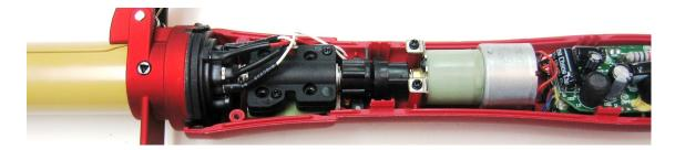
32. The following image of a dismantled Accused Product shows the terminal discs located between the bearing and the cylinder:
