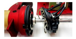
29. The following image of a dismantled Accused Product shows that the first terminal disc is held adjacent to the second terminal disc so that the contacts of the first terminal disc remain in contact with the contacts of the second terminal disc to provide an electrical circuit across the contacts to the heating element in the cylinder:
