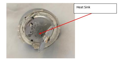
(photograph of Halco Chandelier Light with outer glass bulb and inner reflector removed, showing LEDs disposed in heat sink).
