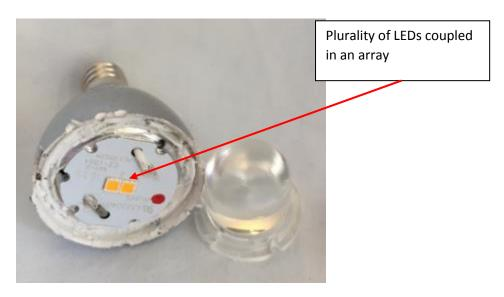
(photograph of Halco Chandelier Light with outer glass bulb and optic removed, showing LED array).
