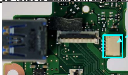
Toshiba R930 Audio PCB (Side A Enlarged), Highlighting Speaker Connector
