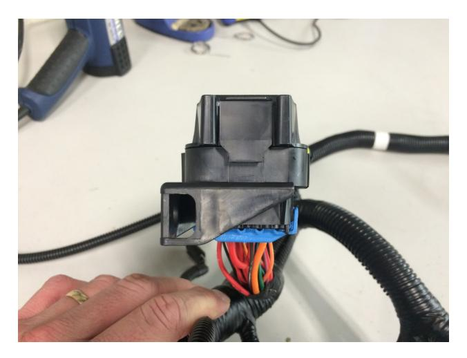
22. The power distribution module in the Sportsman 570 ATV includes "a plurality of electrical components each having at least two leads inserted into the upper receivers of the component receptacles." (*Id.*, Col. 8, Il. 63-65.) The following photographs of components of the Sportsman 570 ATV show the electrical components having at least two leads inserted into the upper receivers of the component receptacles.
