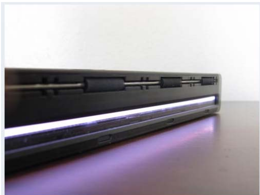
Bottom of the unit sports a set of roller wheels and the scanning light. The scanning light only operates when the roller bar is turning (and of course, when the unit has been powered on and the scan start button has been pressed). This photo was taken by spinning the roller bar outside of the camera's view.
