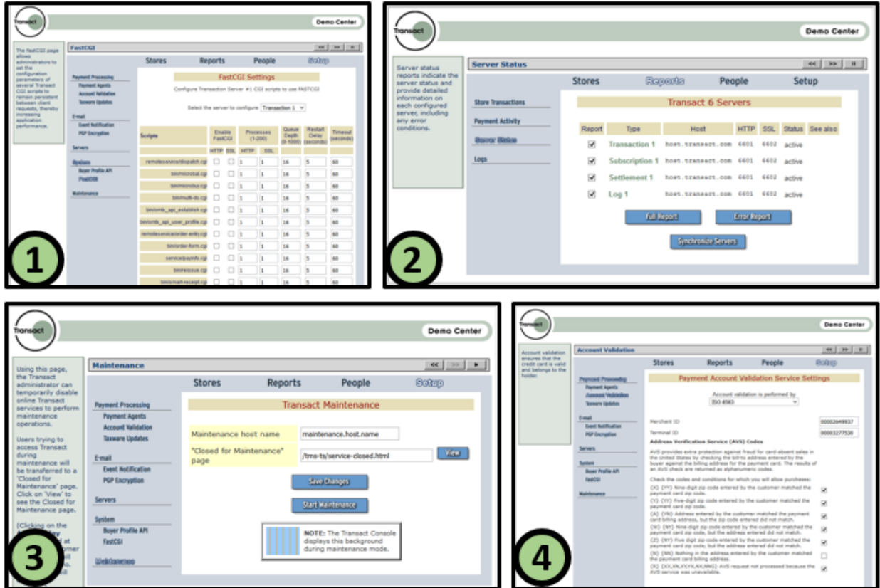
A COLLECTION OF IMAGES OF THE OPEN MARKET TRANSACTION SYSTEM (the numbered annotations correspond to the (1) FastCGI settings, (2) server status screen, (3) Transact maintenance settings, and (4) account validation settings).
