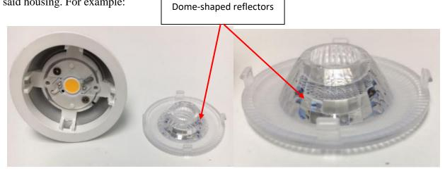
(photographs of Great Eagle 8W MR16 GU10 Bulb, showing dome-shaped reflector optic and LED array it is positioned above, and of dome-shaped reflector itself).
