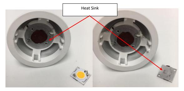
(front and reverse photographs of Great Eagle 8W MR16 GU10 Bulb with outer optic removed, showing LEDs disposed in heat sink).
