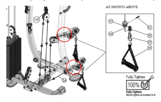
(HTX-2000 Owner's Manual at 25 (red circles added to highlight cable connections to cable stopper shells 37).)
