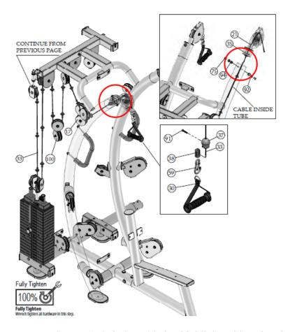
(HTX-2000 Owner's Manual at 24 (red circles added to highlight cable exit point).)
