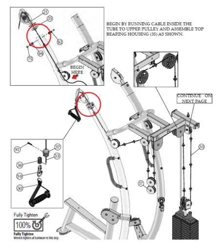
(HTX-2000 Owner's Manual at 23 (red circles added to highlight cable exit point).)
