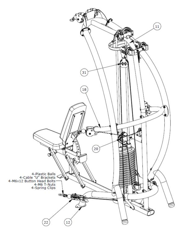
(M1 Inspire Assembly & Operation Manual at 19 (showing plastic balls, cable "U" brackets, M6x12 button head bolts, and M6 T-nuts).)
