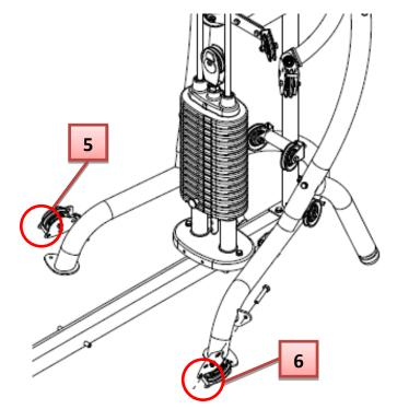
(M1 Inspire Assembly & Operation Manual at 14 (red circles highlighting cable exit points).)
