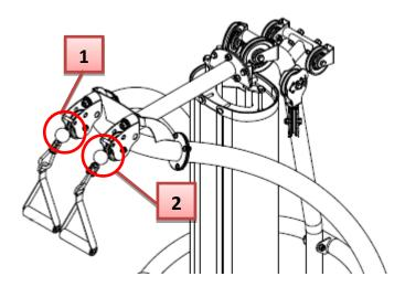
(Ex. B, hereinafter "M1 Inspire Assembly & Operation Manual," at 21 (red circles highlighting cable exit points).)
