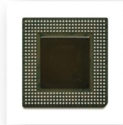
10. A ball grid array is a type of surface-mount packaging (a chip carrier) used for integrated circuits. BGA packages are used to permanently mount devices such as microprocessors. A BGA can provide more interconnection pins than a dual in-line or flat package.
