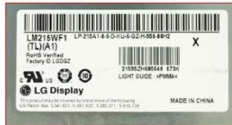
LG LCD Module, LM215WF1 used in Lenovo L215wA Full HD LCD Monitor
