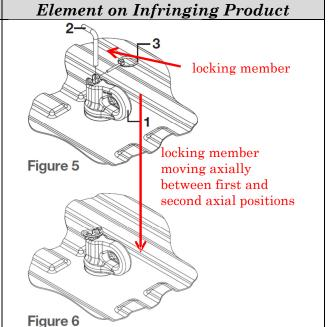
The locking member, when in second axial position, prevents the body member from rotating within the receiving member:
