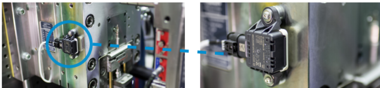
Application Example: Condition Monitoring at an Injection Molding Machine in harsh environment
