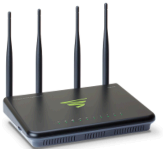
Figure 1. The XWR-3100 is compliant with IEEE 802.11ac and 802.11n wireless distribution systems, and therefore provides a customer premises system.
