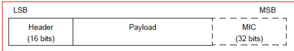
Figure 2.12: Data Channel PDU
