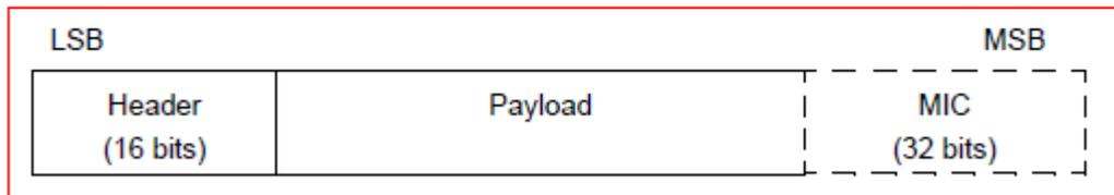
Figure 2.12: Data Channel PDU
