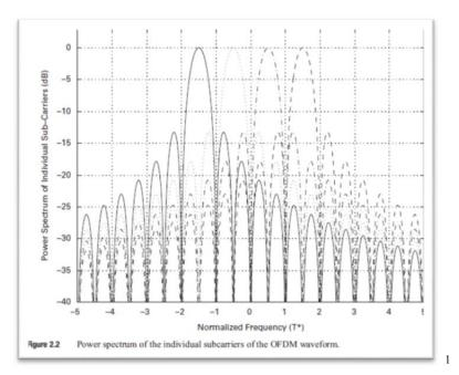
40. OFDM systems contain individual subcarriers that are orthogonally spaced apart in the frequency domain such that they do not interfere with each other as shown in the figure
