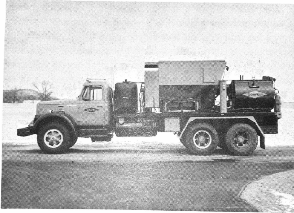
Fig. 8.9 Two-shaft gas turbine engine driving a positive displacement pump.
