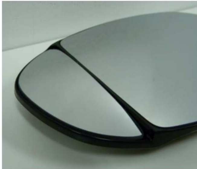
Figure 18 – SMR Fiat 500 Reflective Elements
