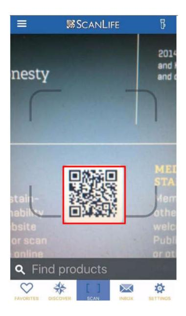
15. As illustrated below, a photographic image of the code pattern is obtained using a camera of the user terminal (e.g., the camera of the smartphone). A processor of the user terminal processes the photographic image of the code pattern to extract the code pattern from the photographic image. The extracted code pattern is decoded by the processor into code information (e.g., the URL of the web page associated with Defendant).
